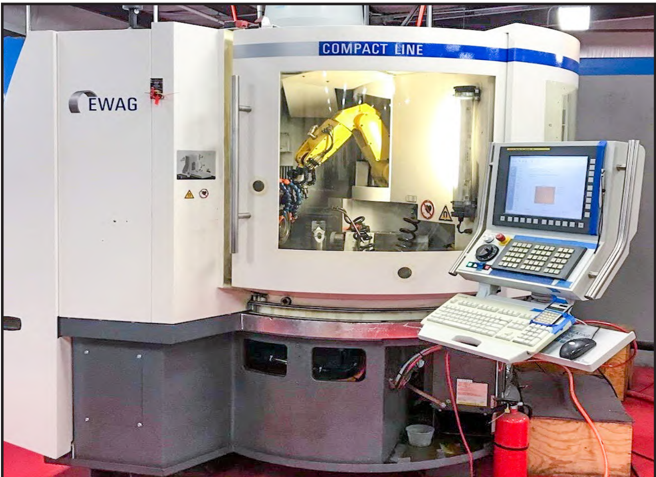
Our second EWAG CNC Tool and Cutter Grinder with Robotic Loader. December 2018
