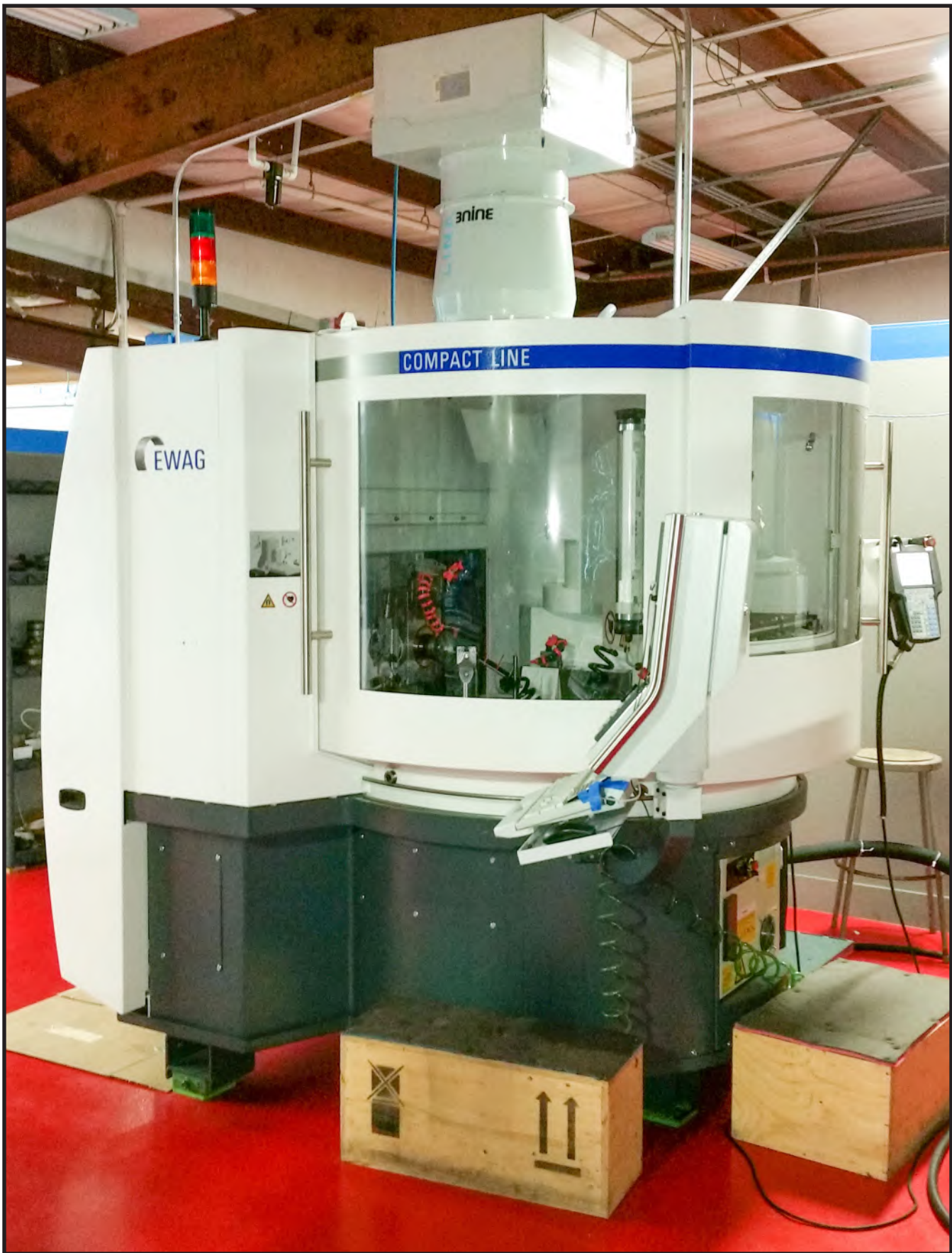
Carbide Grinding's first CNC Tool and Cutter Grinder with Auto-Loading Robot, 2014.
